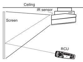
b) RCU used in a hardwired configuration.
